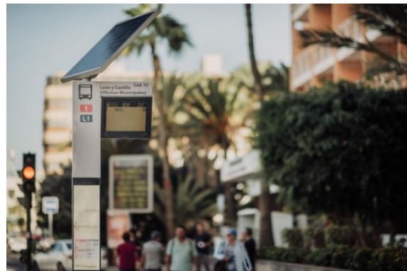
Figure 1: Real time information panel powered by solar energy
